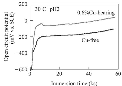
Fig. 4 Effect of Cu addition on the open circuit potential of 21%Cr-0.3%Ti stainless steels
