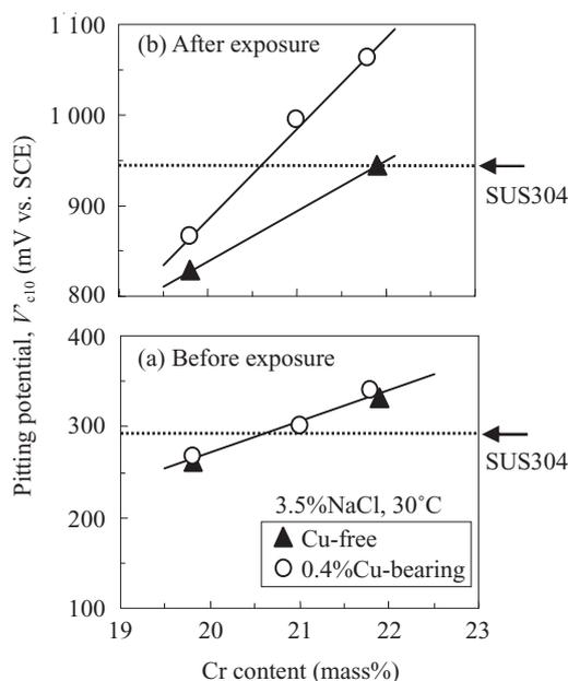
Fig. 1 Effect of Cr content and Cu addition on the pitting potential of 20–22%Cr-0.3%Ti stainless steels before or after 1.5 years field exposure (The pitting potential before and after exposure was measured by polished surface and as-exposed surface, respectively.)
