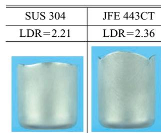
Photo 3 Comparison of Limiting Drawing Ratios between JFE443CT and SUS304 (Thickness of specimen 0.8 mm)
