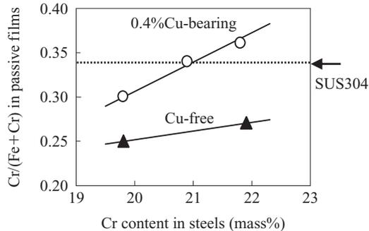
Fig. 2 Effect of Cr content and Cu addition on the ratio of Cr to Fe+Cr in passive films formed on 20–22%Cr-0.3%Ti stainless steels after 1.5 years field exposure
