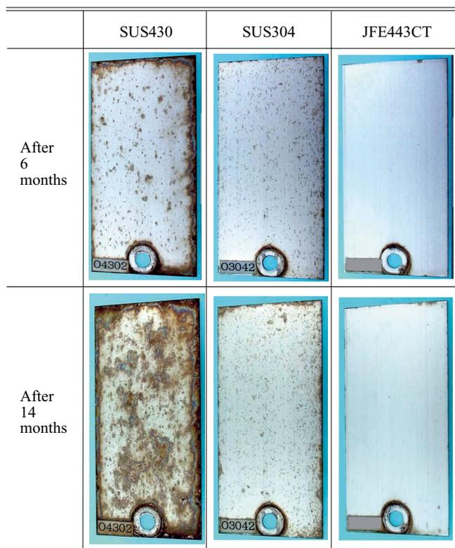
Photo 2 Appearance of JFE443CT, SUS304, and SUS430 after 6 and 14 months field exposure test in a coastal area at Okinawa (#800 surface finished, Sample size: 75 × 150 mm)
