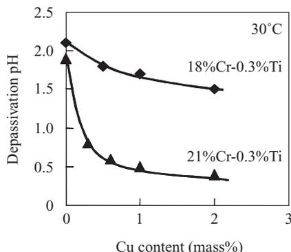
Fig. 3 Effect of Cu addition on the depassivation pH of 18%Cr-0.3%Ti stainless steels and 21%Cr-0.3%Ti stainless steels
