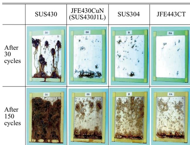
Photo 1 Appearance of various stainless steels after JASO M 609-91 (JASO: Japanese Automobile Standards Organization) mode cyclic corrosion test (#600 polished surface, Sample size: 60 × 80 mm)
