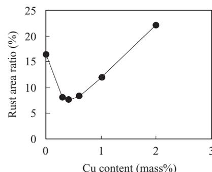
Fig. 5 Influence of Cu content on the rust area ratio of 20%Cr-0.3%Ti stainless steels after one month exposure
