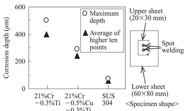
Fig. 6 Effect of Cu addition on the crevice corrosion depth of 21%Cr-0.3%Ti stainless steels after 90 cycles JASO M 609-91 mode cyclic corrosion test (JASO: Japanese Automobile Standards Organization)
