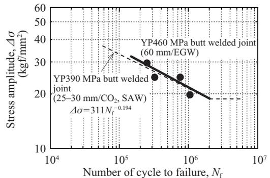
EGW: Electrogas arc welding SAW: Submerged arc welding
