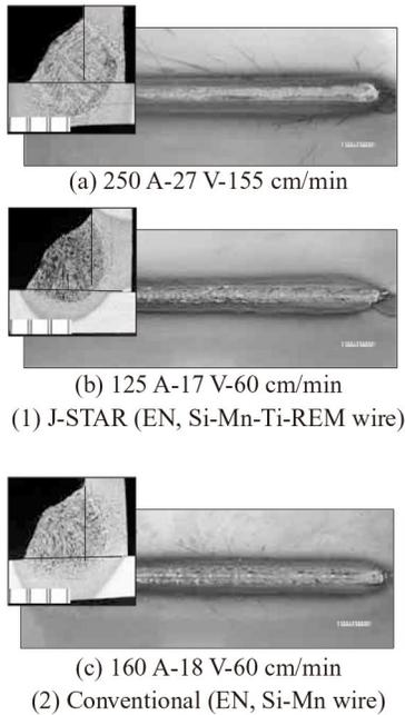
Fig. 2 Welding bead appearance and cross-sectional macroscopic organization
