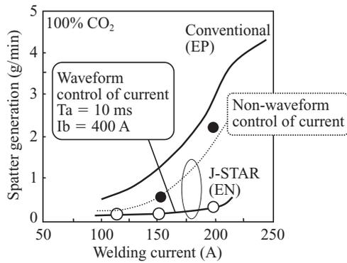
Fig. 5 Relationship between welding current and spatter generation
