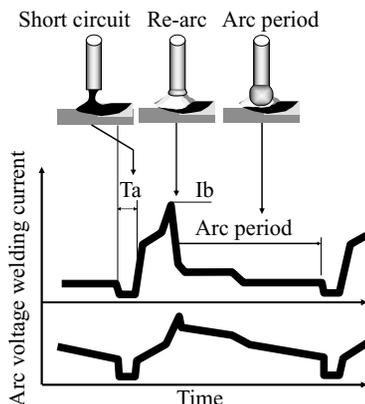
Fig. 3 Waveform control of welding current
