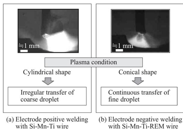
Fig. 1 Arc phenomena in CO<sub>2</sub> gas shielded arc welding
