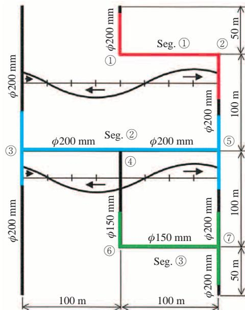
Fig. 5 Distribution network model for verification of NeEX
