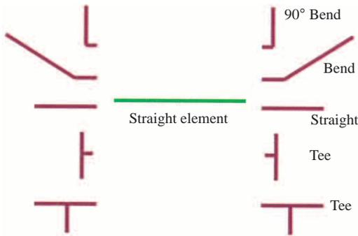
Fig. 2 Definition of segments to idealize distribution network
