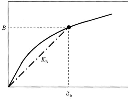
Fig. 4 Force-displacement relation of a boundary element
