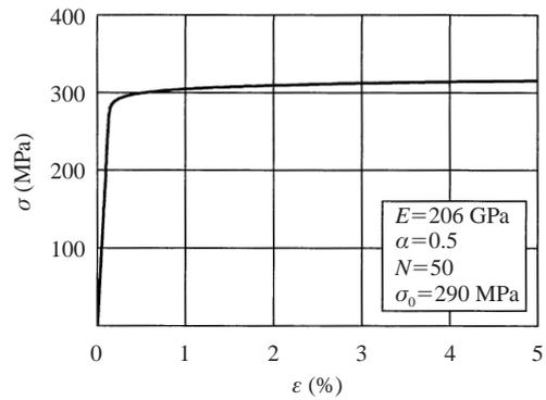
Fig.7 Stress strain relationship of pipes
