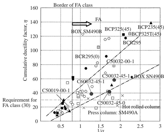
Fig.5 Relationship between cumulative ductility factor,  $\eta$  and general width-thickness ratio,  $a$
