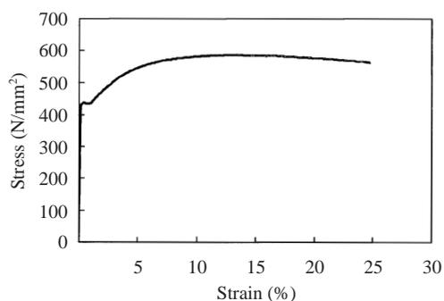
Fig.1 Stress-strain relationship ( $t = 32$  mm)
