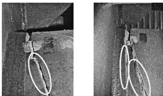
Photo 1 Fracture parts
