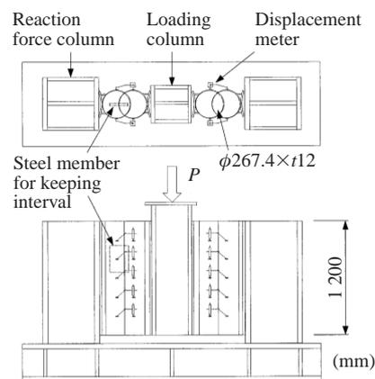
Fig. 5 Pipe-junction shear test specimen
