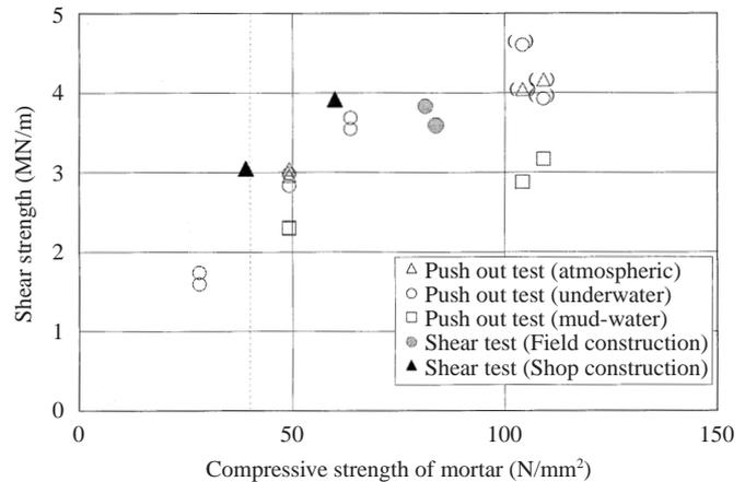
Fig. 8 Relation of shear strength and compressive strength
