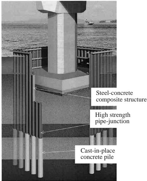
Fig. 2 Schema of Hyper-Well-SP (with Cast-in-place-concrete pile)
