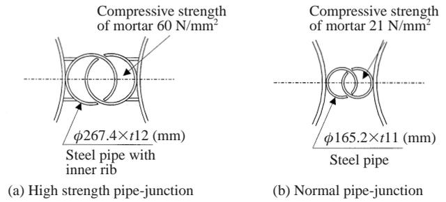
Fig. 3 Dimension of high strength pipe-junction
