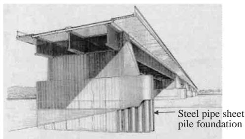
Fig. 12 Pier foundation (standing style)
