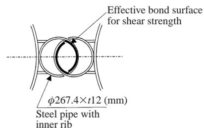
Fig. 9 Effective bond surface for shear strength
