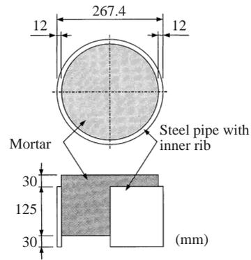
Fig. 7 Test specimen for push out test
