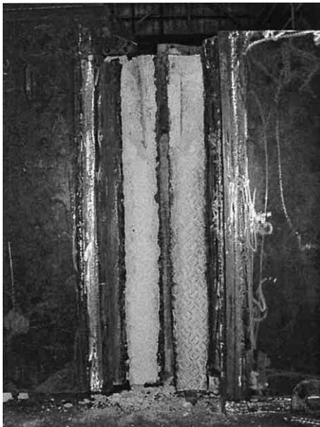
Photo 2 Appearance of mortar filling (Test specimen 1)
