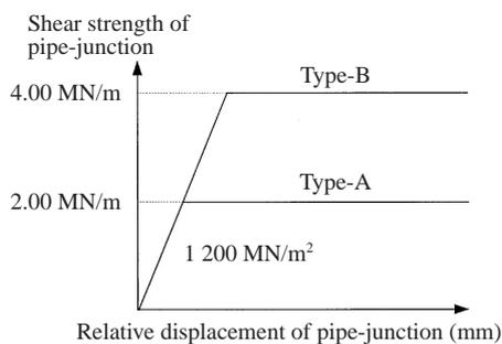
Fig. 10 Analysis model for shear character of pipe-junction
