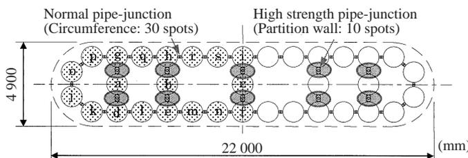
Fig. 13 Cross section of steel pipe sheet pile foundation
