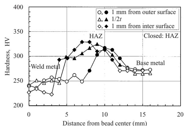
Fig.3 Hardness distribution in the welding joint
