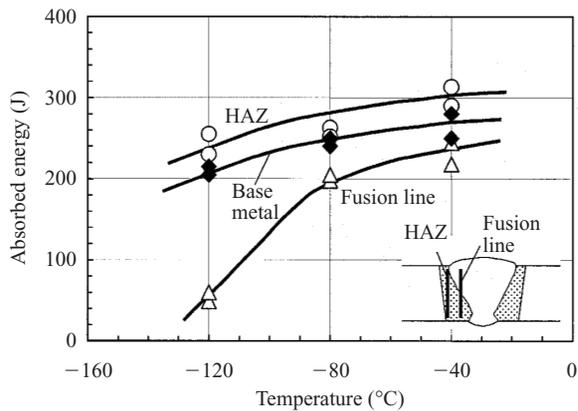
Fig.4 Relationship between Charpy absorbed energy and temperature
