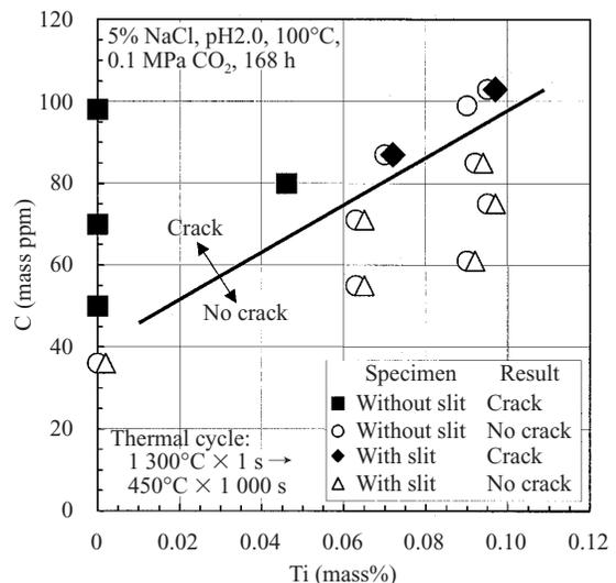
Fig.9 Effects of C and Ti on SCC test results
