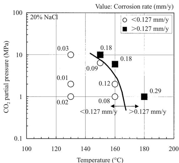
Fig.5 CO<sub>2</sub> corrosion test results of the base metal
