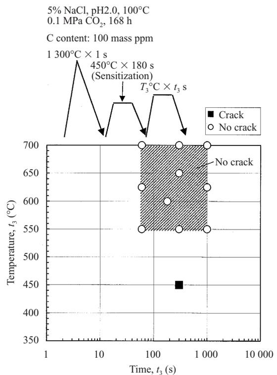
Fig.8 Effects of thermal cycle conditions after sensitization on SCC behavior
