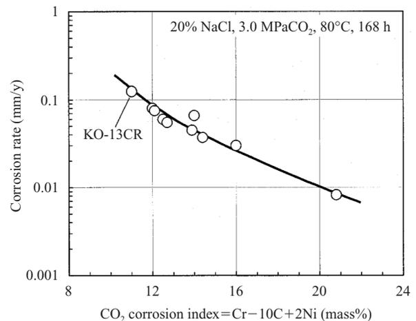
Fig. 1 Relationship between corrosion rate and CO<sub>2</sub> corrosion index
