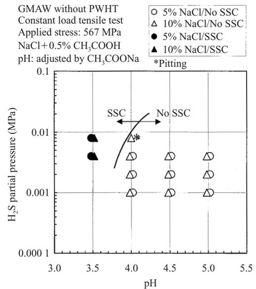
Fig.6 SSC test results of the welded joint
