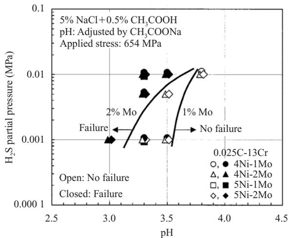
Fig.2 Effects of Ni and Mo on SSC resistance of 0.025C-13Cr steels
