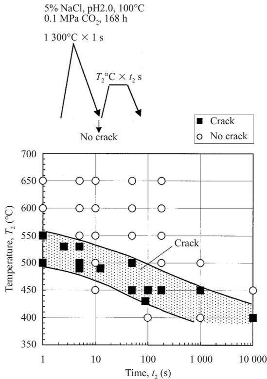
Fig.7 Results of U-bend SCC tests for simulated HAZ
