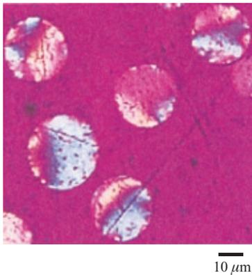
Photo 1 Polarized micrograph of mesophase spheres formed in coal-tar pitch
