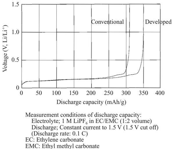
Fig. 3 Discharge capacity of developed and conventional KMFC graphite powders
