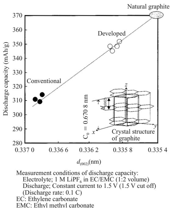
Fig. 4 Relation between  $d$ -spacing  $d_{(002)}$  and discharge capacity of developed and conventional KMFC graphite powders
