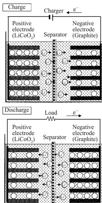
Fig. 1 Principle of the lithium ion secondary battery
