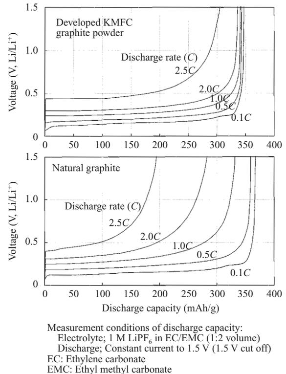
Fig. 5 Comparison in discharge rate property of developed KMFC graphite powder and natural graphite powder
