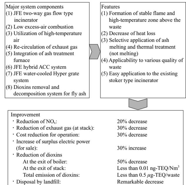
Fig. 1 Expected effect of advanced stoker system
