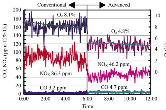
Fig.9 Changes in O<sub>2</sub>, CO and NO<sub>x</sub> in flue gas with time
