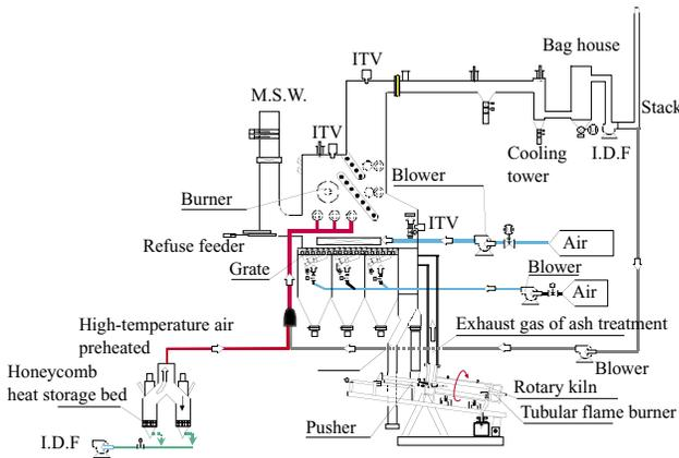
Fig.4 MSW incineration test plant of pilot scale
