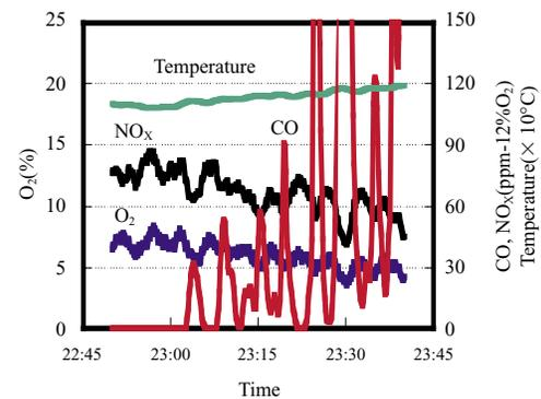
Fig.5 Changes in O<sub>2</sub>, CO, NO<sub>x</sub> and gas temperature with time in test plant under conventional combustion at  $\lambda = 1.3$
