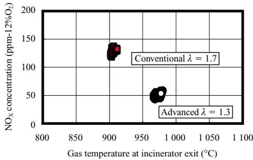
Fig. 7 NO<sub>x</sub> concentrations at incinerator exit in test plant
