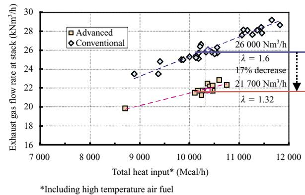
Fig.11 Relationship between total heat input and exhaust gas flow rate at stack
