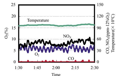
Fig.6 Changes in O<sub>2</sub>, CO, NO<sub>x</sub> and gas temperature with time in test plant under advanced combustion at  $\lambda = 1.3$
