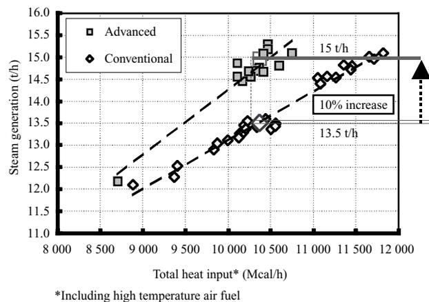
Fig.12 Relationship between total heat input and steam generation
