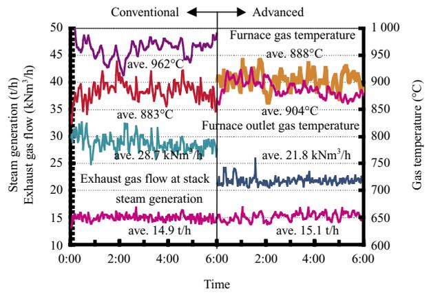
Fig.10 Changes in steam generation, exhaust gas flow rate and gas temperatures with time
