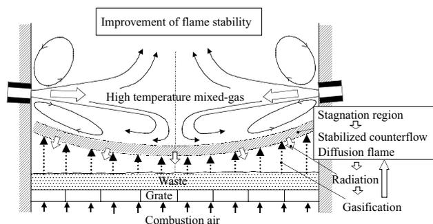
Fig.3 Flame stabilization image in the combustion beginning region
