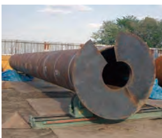
Toe wings and a construction method of the JFE Tsubasa Pile™
