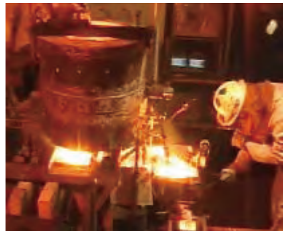
Molten steel casting experiment using small scale continuous casting simulator
