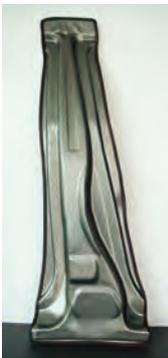
UHSS structural part (Center pillar: 1180MPa steel)
