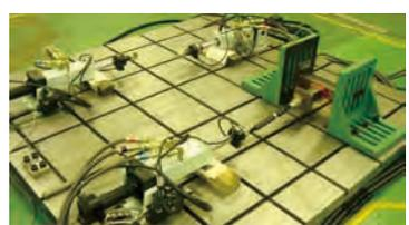
Tri-axial fatigue testing machine
