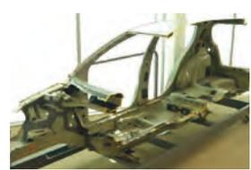
Disassembled half body
