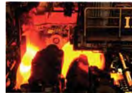
Sheet bar coiler Sheet bars are coiled to prevent temperature drop.
