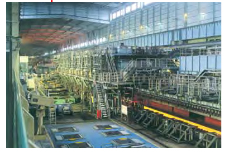
Finishing mill The finishing mill rolls the arriving sheet bars to the specified thickness
