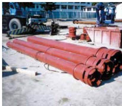
Pilers (Pile head rotation type)
