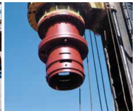
Cap (Pile head rotation type)
