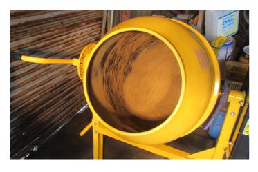
1. Blade of concrete mixer should be removed before iron-coating.
