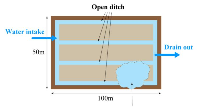
Seed would be died in continuous flooded area. ⇒ Open ditch helps to drain water easily.
