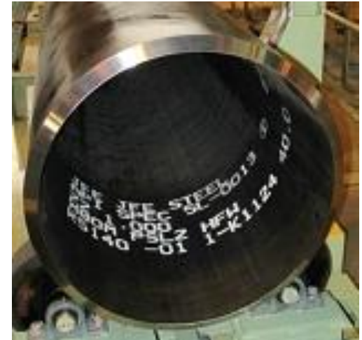
World thickest X80 HFW pipe X80 559 mm (22") x 25.4 mm (1.000")
