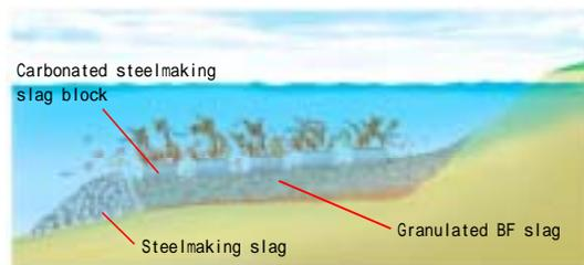
Fig.5 Scheme of demonstration test using iron and steelmaking slag and blocks
