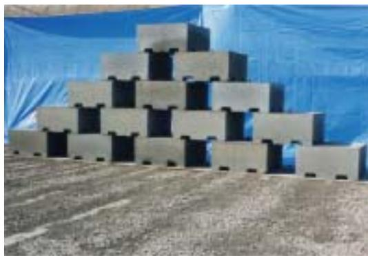
Photo 5 A pile of steelmaking slag blocks
