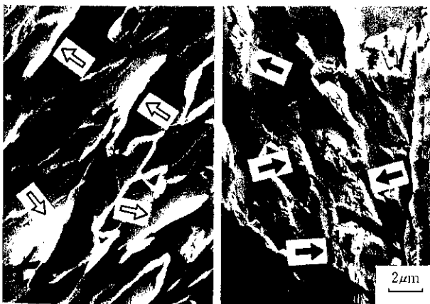
(a) ICCG HAZ (⇨ M-A constituents) (b) ICCG HAZ tempered at 450°C (⇨ Ferrite-cementite aggregates)
