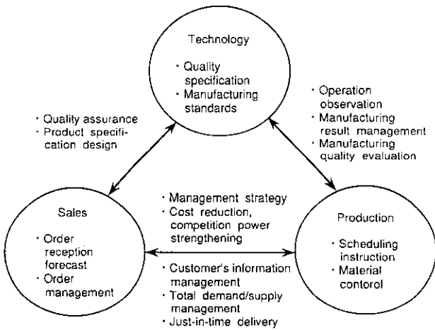
Fig. 1 The structure and aim of computer integrated manufacturing (CIM) system for iron powder
