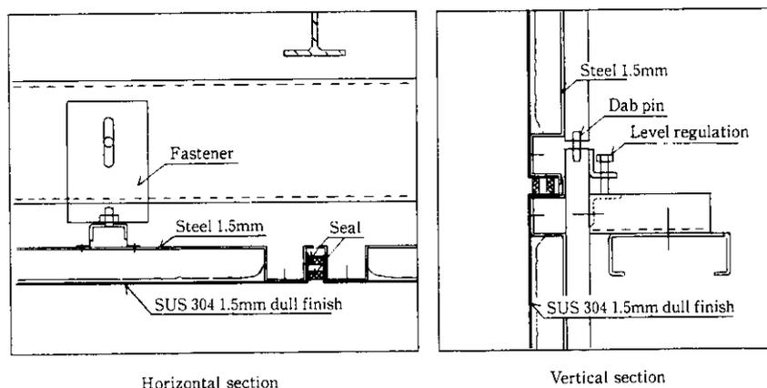
Fig. 3 Standard panel section of exterior wall
