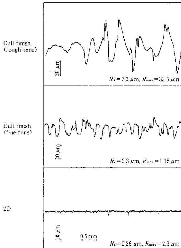
Fig. 1 Surface profile of dull-finished stainless steel sheet (longitudinal direction)
