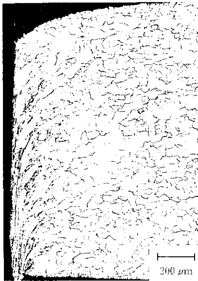
Photo 1 Microstructure and metal flow at the punched hole in EFE-3AD
