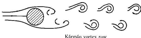
Fig. 2 State of vortices behind a round column
