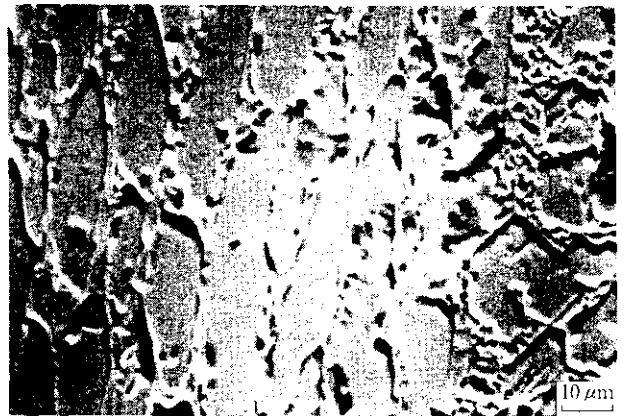
Photo 3 Micro structure of ceramic composite metal (Cobalt alloy + ceramics)
