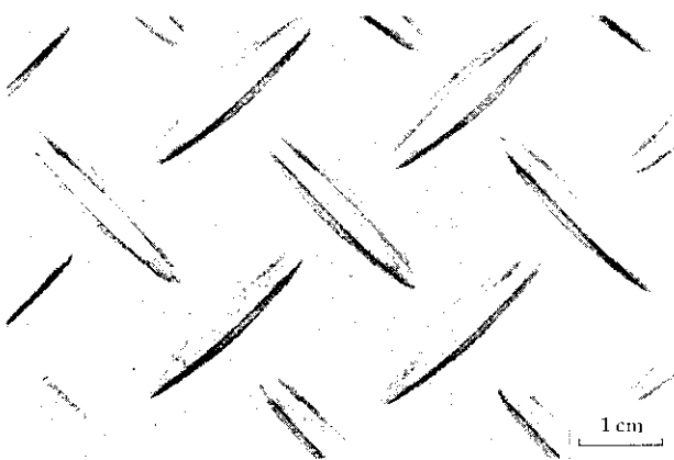
Photo 2 Appearance of SUS 304 floor plate
