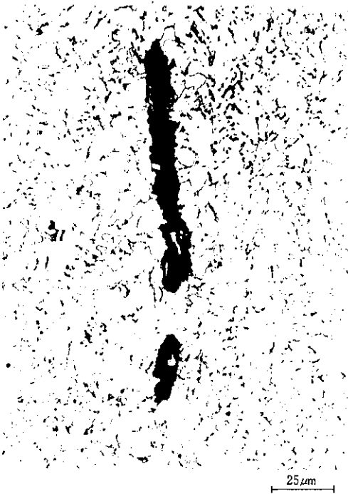
Photo. 8 Micrograph of penetrator (nital etching)
