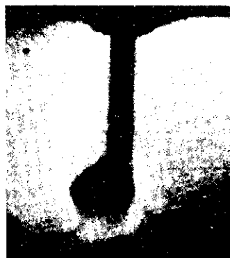
Photo. 1 Pendant metal drop at a wire tip during arcing period of short-circuit transfer welding on the plate contained 0.021%RE
