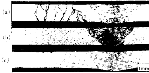
(a) : Stress corrosion cracking (b) : Pit formed due to the intergranular corrosion at welded zone (c) : Pitting corrosion
