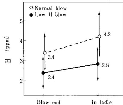
Fig. 4 Effectiveness of low hydrogen LD blowing
