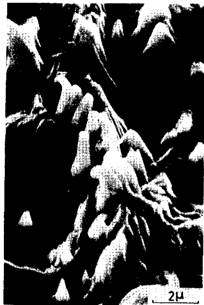
Photo. 4 Scanning electron micrograph of the center of crater produced by rastering \text{Ar}^+ ion beam bombardment (dose 1.1 \times 10^{19} ions/cm 2 )
