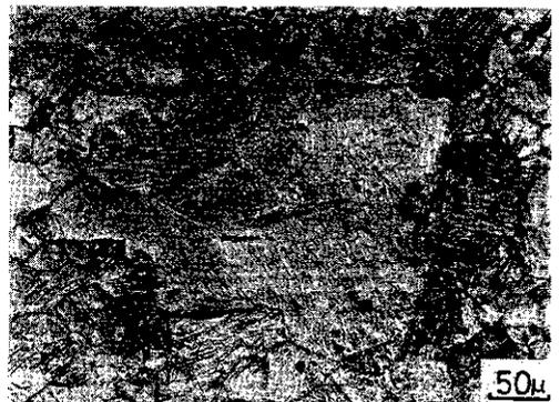
**Photo. 4** A coarse grain produced by reheating to 1150°C and 6% rolling at 900°C in Nb-steel
