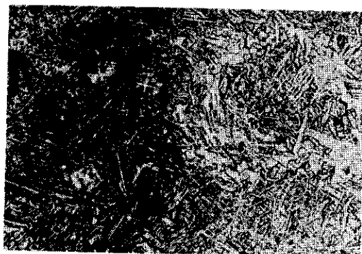
Photo. 11 Microcrack observed in the vicinity of type III crack \times 400 \left( \times \frac{7}{10} \right)
