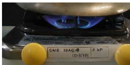
(b) 13A specification, damper opening : 8/10
