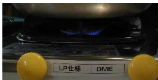
(a) LPG specification, damper opening : fixed
