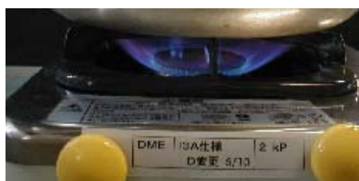
(c) 13A specification, damper opening : 5/10
