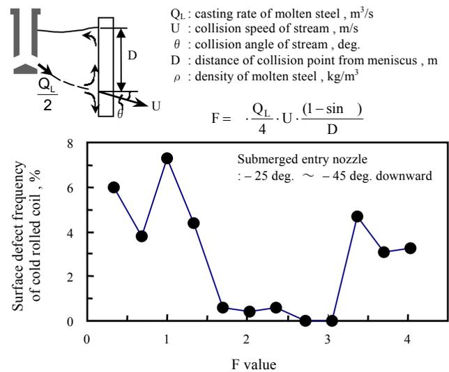
**Fig.1** Relationship between F value and surface defect frequency on cold rolled coil<sup>1)</sup>
