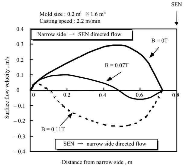
**Fig.10** Calculated profile of meniscus flow velocity along mold width direction at different EMLS intensities
