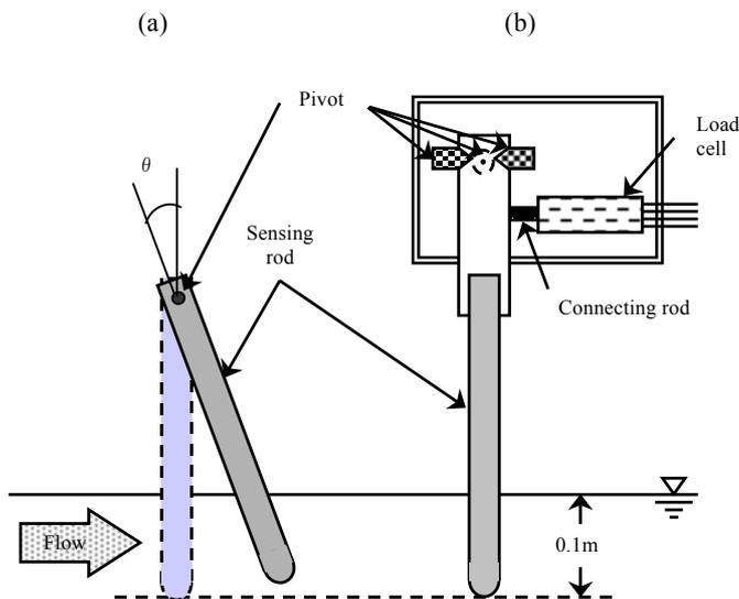
**Fig. 6** Schematic illustration of devices for meniscus flow tachimetry
