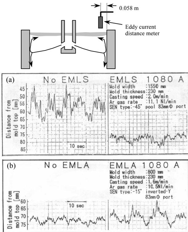
**Fig. 5** Change of meniscus level fluctuation in the vicinity of narrow side of mold by EMLS and EMLA
