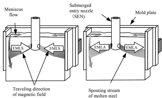
**Fig.2** Driving force imposed upon molten steel by EMLS and EMLA
