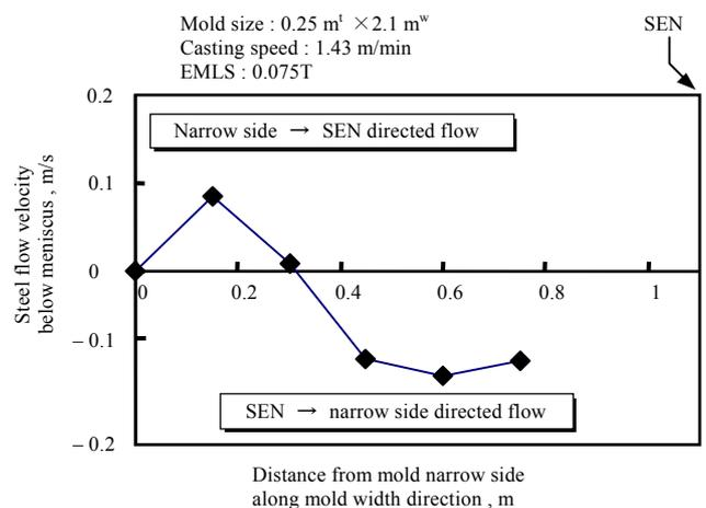
**Fig.11** Measured profile of meniscus flow velocity
