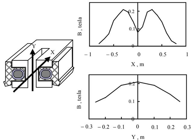
**Fig.4** Magnetic field profile of the traveling magnetic field generator
