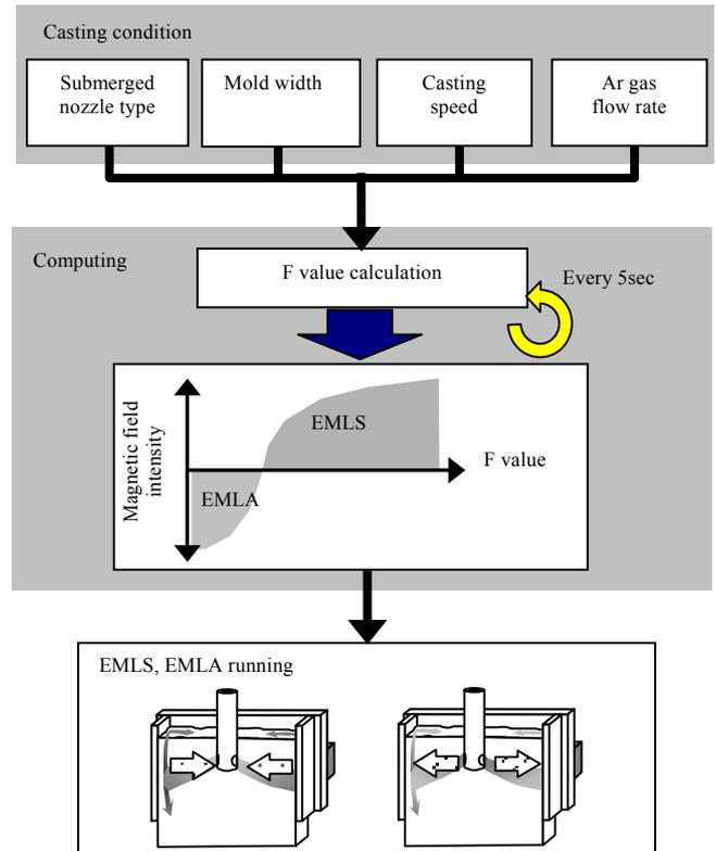
**Fig.15 Schematic diagram of computer control of EMLS and EMLA**
