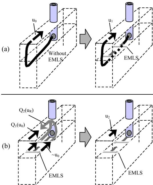
**Fig.12 Schematic illustration of meniscus flow braking mechanism by EMLS**
