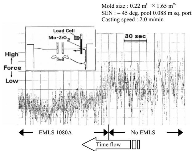
**Fig. 7** Time-series change of meniscus flow velocity by EMLS
