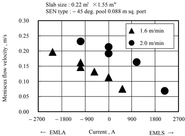
**Fig.8** Change of time-averaged meniscus flow velocity in the vicinity of narrow side of mold by EMLS and EMLA at various intensities
