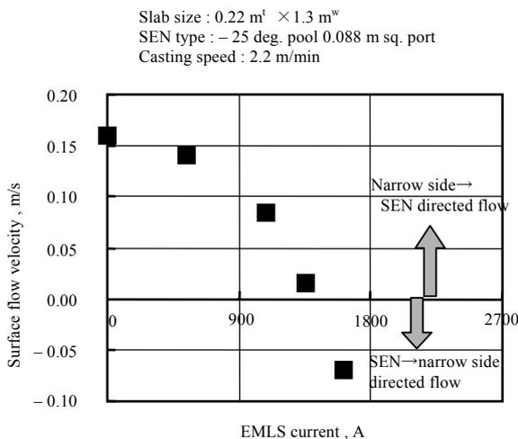
**Fig.9** Change of time-averaged meniscus flow velocity at quarter-width point by EMLS and EMLA at various intensities
