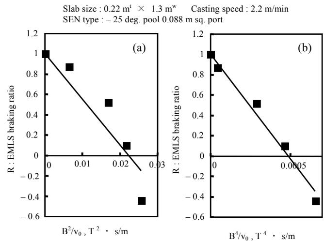
**Fig.13 Relationship between EMLS braking ratio and two parameters for analyzing EMLS effect**
