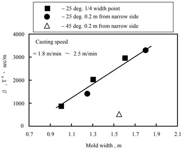
**Fig.14 Relationship between mold width and coefficient of EMLS braking effect,  $\beta$**
