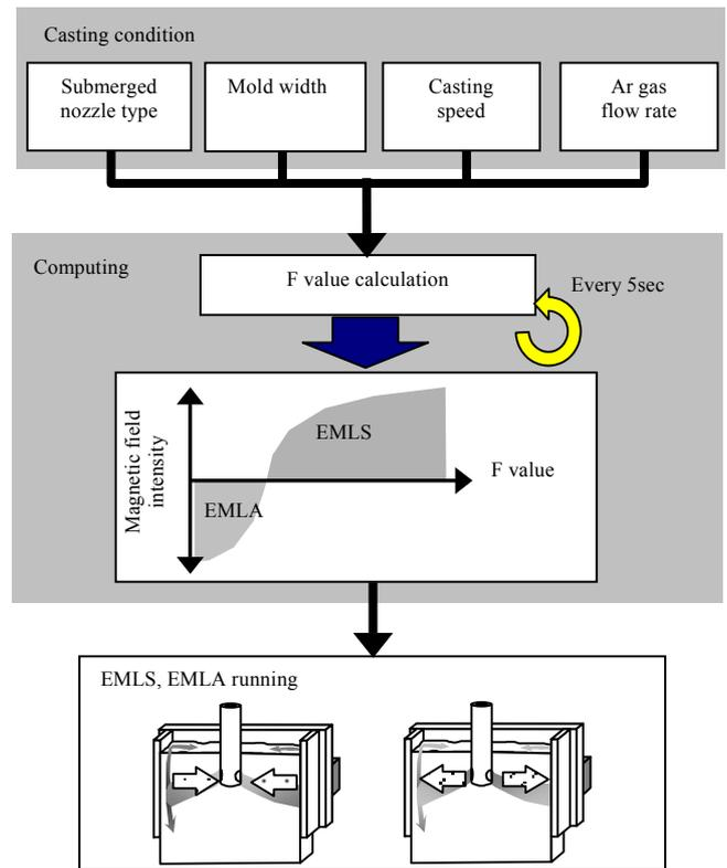
**Fig.15 Schematic diagram of computer control of EMLS and EMLA**
