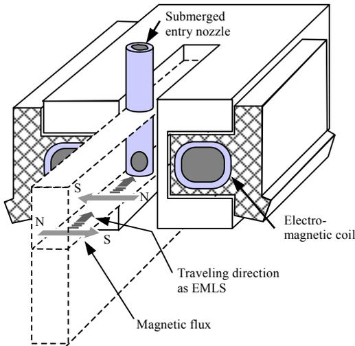
**Fig.3** Schematic illustration of installation of the magnetic field generator for EMLS and EMLA
