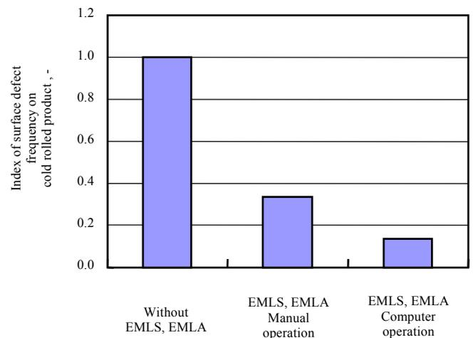
**Fig.16 Effect of EMLS and EMLA on product surface defects**
