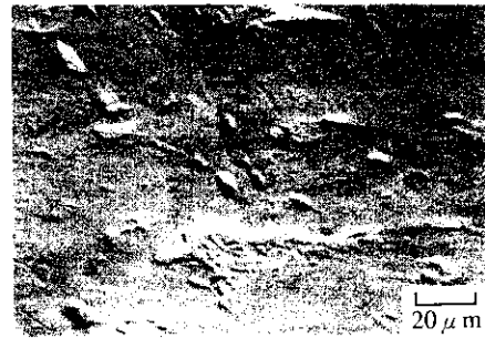
Photo 2 SEM images of wear surface of HSS type alloyed steel after hot wear test disk
