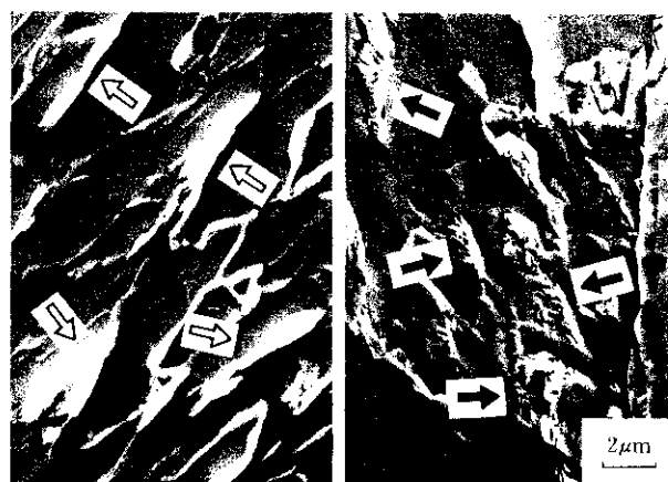
Photo 1 Scanning electron microscopic observation of simulated HAZs
