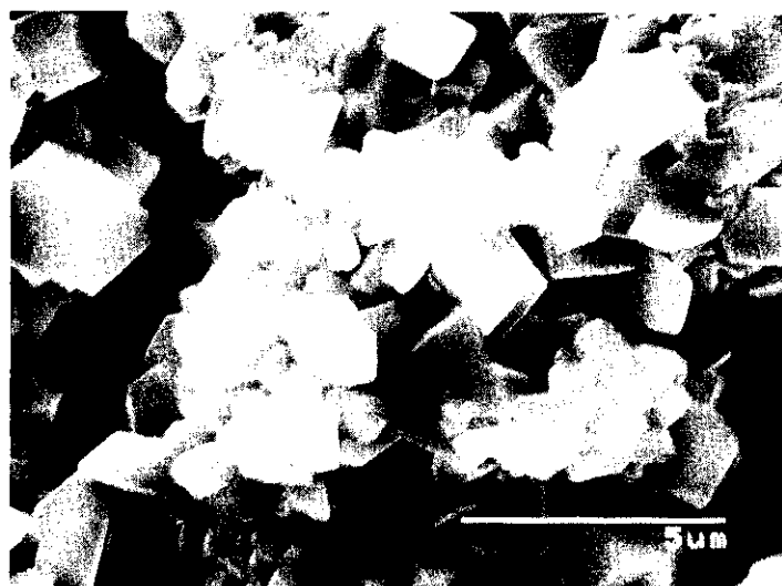
Photo 1 \text{Cr}_2\text{O}_3 on the surface of RF-100 sheet
