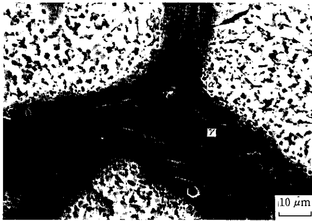
Photo 5 A SEM observation of an oxalic acid etched specimen (PT = 1350°C, water quenched)
