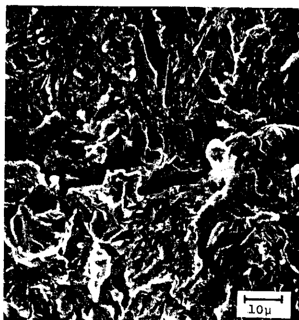
Photo. 4 Scanning electron micrograph of the fractured surface of the straight crack
